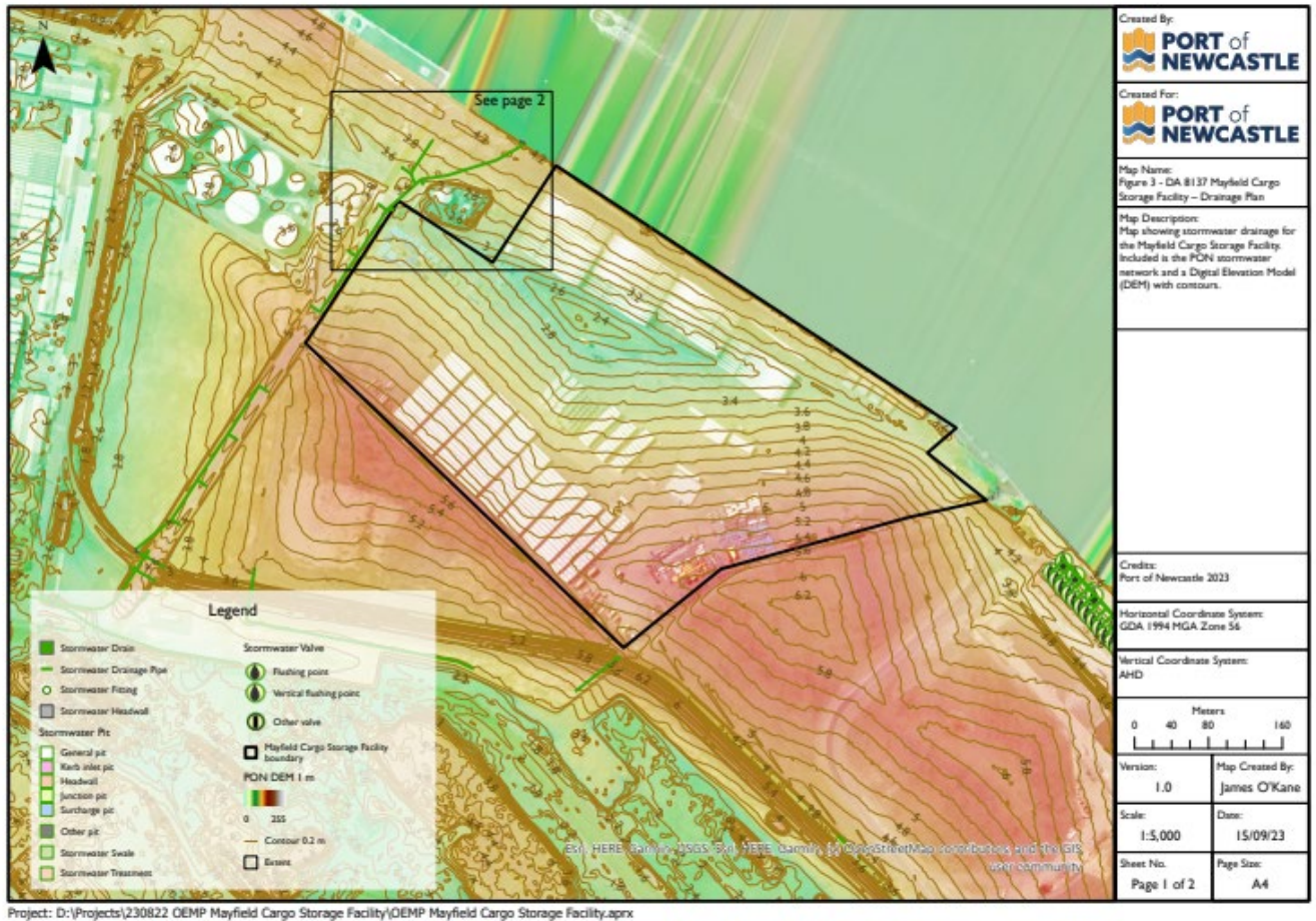
Figure 4: Drainage Plan for DA 8137 Cargo Storage Facility
