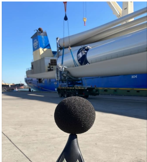
Measurement of crane operations during unloading of wind turbine blade
