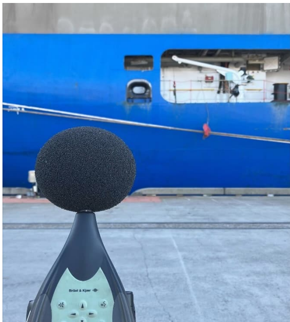
Measurement of vessel engine noise
