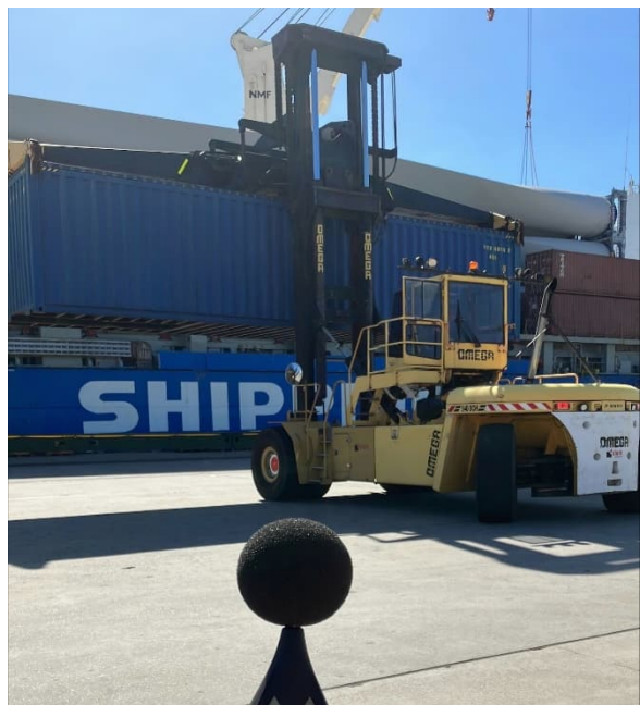
Measurement of container handler lifting and moving container
