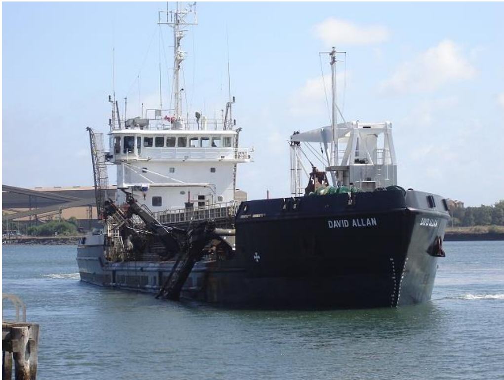
Figure 4 The David Allan trailing suction hopper dredger
