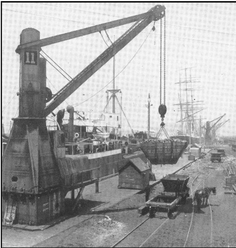
Plate 15: Hydraulic Power Crane. One of the three hydraulic cranes still in operation in 1959. Note the horse to the right of the coal wagon. Port of Sydney, March 1959.
