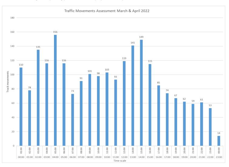
In accordance with Schedule 3, Condition 2.3 of the Mayfield Concept Plan, the following table details truck movements against the prescribed criteria. Note a loaded vehicle is measured as two movements, inward and outward bound of the terminal.
