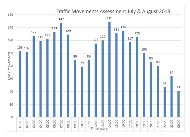
In accordance with Schedule 3, Condition 2.3 of the Mayfield Concept Plan, the following table details truck movements against the prescribed criteria. Note a loaded vehicle is captured as two movements, inward and outward bound of the terminal.
